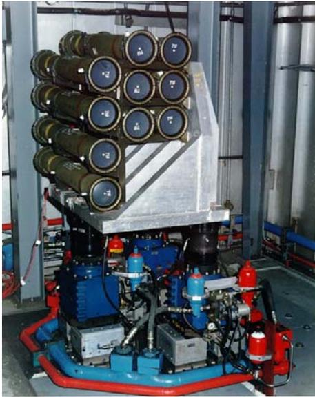
**Figure 1. 3-DOF TOW/M113 Test Configuration**
