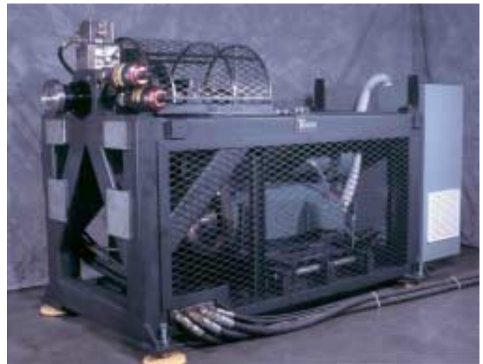
A typical Team Engine Simulation System with integrated variable speed drive.
