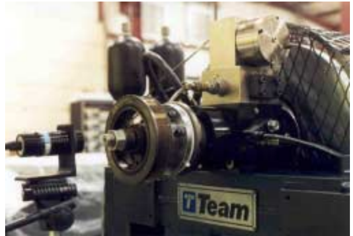
An engine damper test using the Team Engine Simulation System. The sensor on the left is an infra-red temperature sensor.
