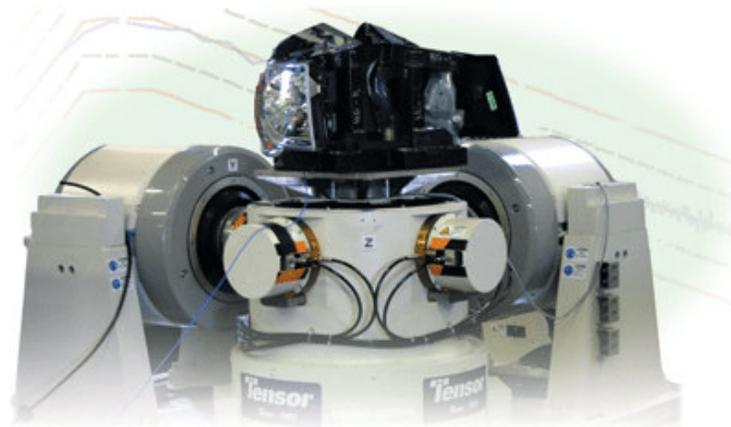
Historically, single-axis, single-shaker testing is the method of choice. Vibration tests are conducted by sequentially applying single-axis vibration to a test article along the product's X, Y, and Z axes. These tests are performed using a linear shaker and rotating the test product to the next axis after each test.
