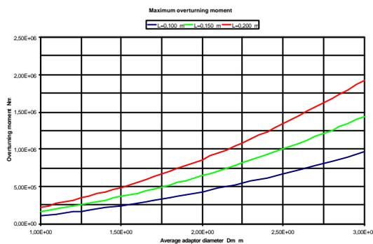
**Fig. 4. Maximum overturning moment capability**
