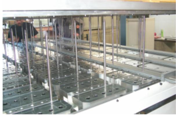
**Fig 7. Table connection alignment tooling**
