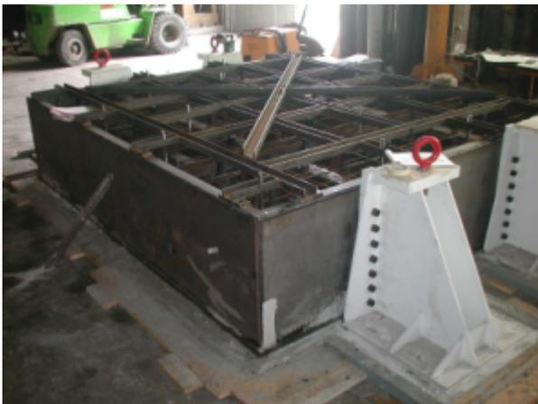
**Fig.6. Steel casing and air cushion steel legs**
