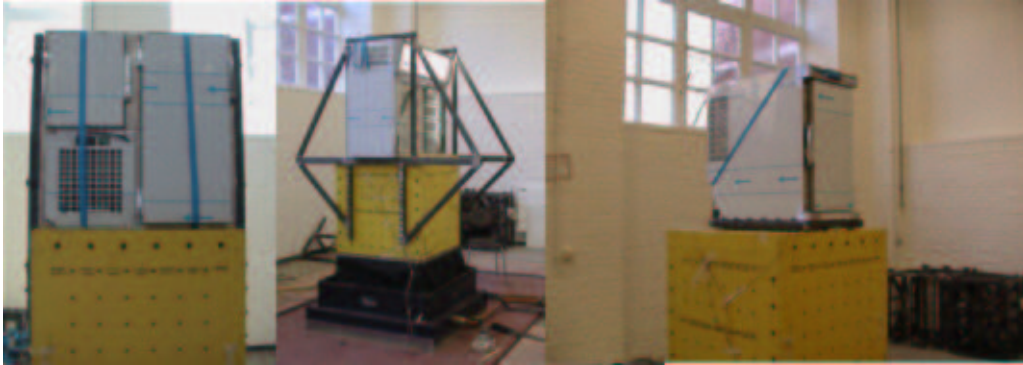
Figure 3 Cube shaker table with some different device setups
