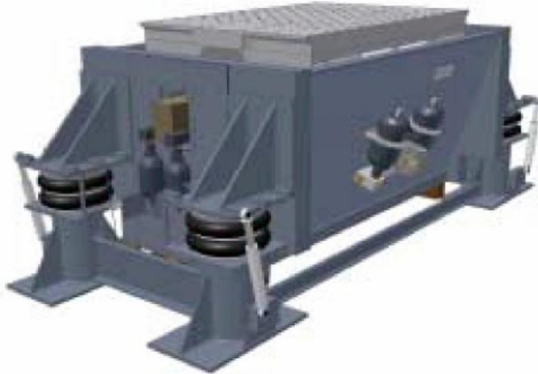
Figure 3.0 Bi-Axial Test System for large payloads
