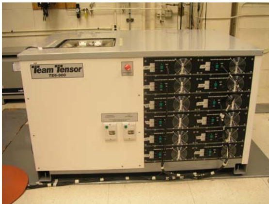
Figure 1. Overview of 6-DOF Shaker System
