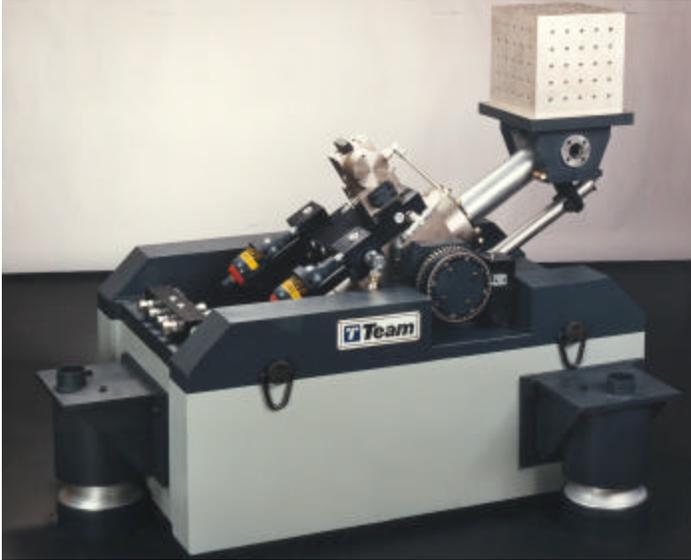
Figure 6.0 Simultaneous bi-axial vibration system used for qualifying small electrical components to IEEE-344.
