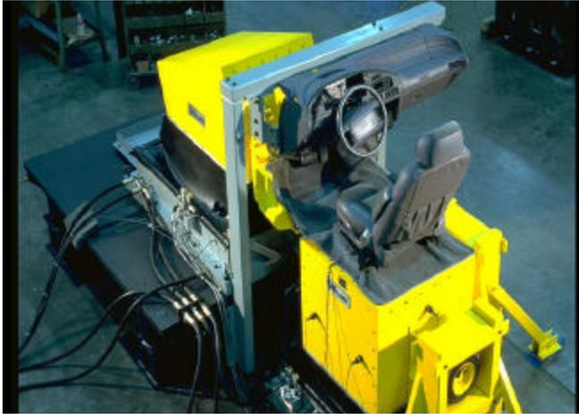
Figure 12.0 Vehicle Vibration Simulator used for subjective evaluation of ride quality. Photo courtesy of the Ford Motor Company.
