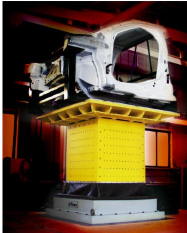
Figure 11.0 Typical automotive durability test set-up using the CUBE. Photo courtesy of MIRA UK
