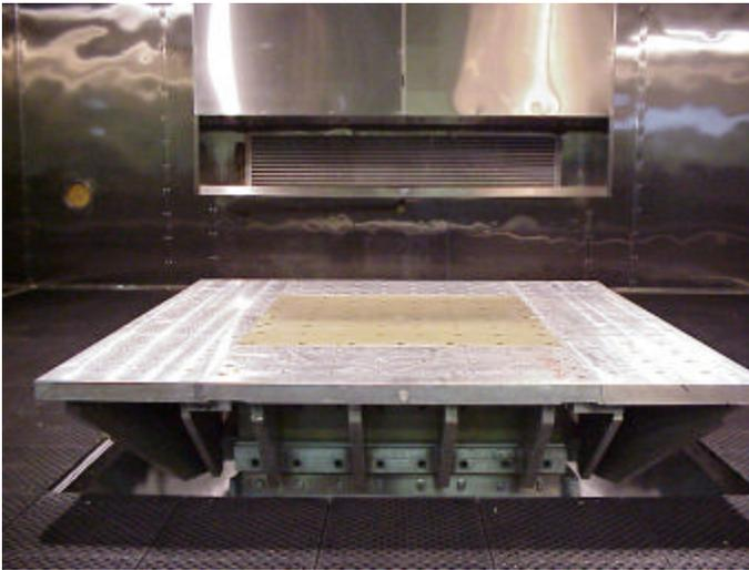
Figure 14.0 CUBE integrated with a thermal chamber. Shows head expander extending into the chamber interior. Photo courtesy of Defiance Labs.
