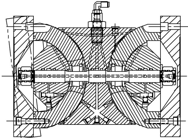
Figure 4.0 Double hydrostatic spherical coupling with +/- 6 degrees of deflection on both ends
