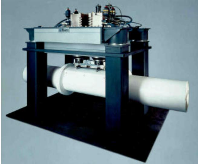
Figure 2.0 Dual Electrohydraulic shaker system driving a mock missile. *Photo courtesy of Northrop Grumman*
