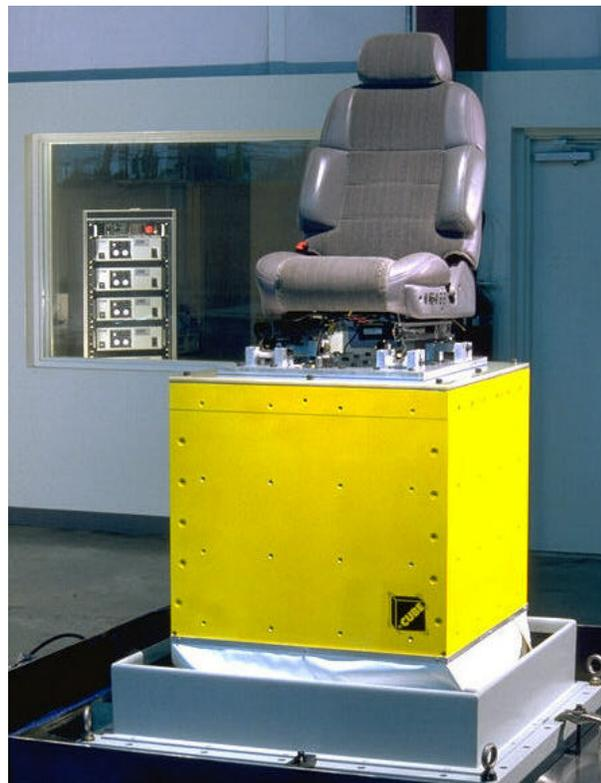
Figure 13.0 Typical car seat mounted on a CUBE. Provides complete access for placement of microphones and other measurement equipment
