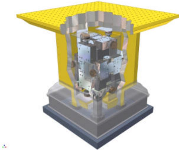
Figure 10.0 Team Corporation CUBE with a 1.5-m square head expander. Interior view shows servohydraulic actuator arrangement.
