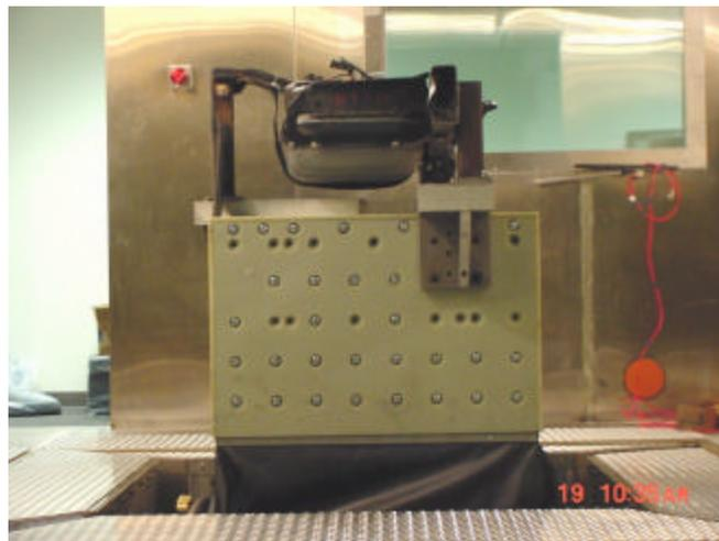
Figure 15.0 Alternate thermal chamber installation of the CUBE. Note the use of G10 epoxy insulation on the entire moving structure. Photo courtesy of Visteon Global Technology Laboratory.
