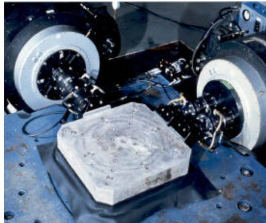
Figure 5.0 Tri-axial vibration system showing two of the three ED shakers and hydrostatic spherical coupling making up the shaker to table connection.
