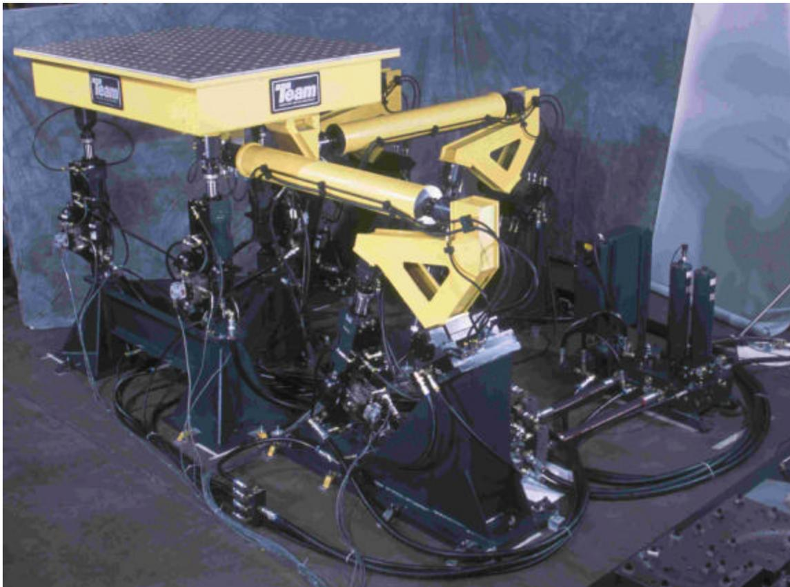
Figure 9.0 Multi Axis Shake Table (MAST) 6 degree of freedom test system. Provides full control of all three translations and three rotations. Normally limited to about  $50 \text{ Hz}$  in maximum frequency response, this table has a higher frequency bandwidth due to the use of hydrostatic bearings throughout.
