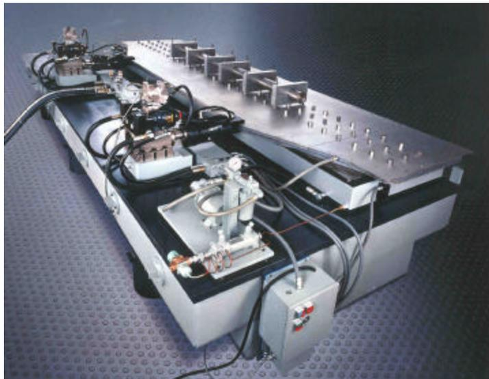
Figure 3.0 Dual shaker horizontal vibration system used for testing oil drill tooling. *Photo courtesy of Schlumberger*
