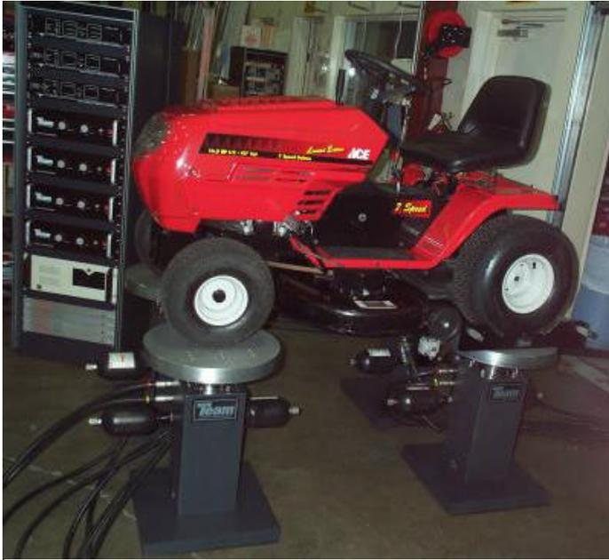
Figure 8.0 Lawn tractor on a small 4-poster servohydraulic test rig. Photo courtesy of MTD
