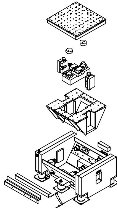
Figure 7.0 True bi-axial vibration system shown in an exploded view. Two vertical actuators flank single horizontal actuator. Other degrees of freedom restrained by hydrostatic planar bearings
