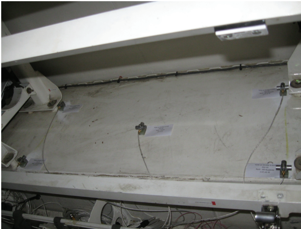
Figure 1. Transducer placement (input to missile rack).
