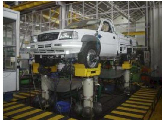
Figure 3- Hydraulic Simulator, from Awate *et al.*, (2007)
