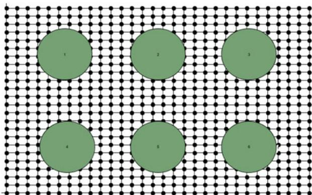
Fig. 5 2D FEA of PWB and inductors, using smearing method
