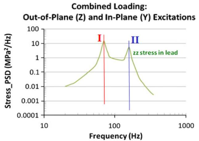
Fig. 13 Stress due to combined loading
