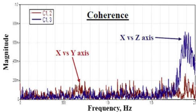
Fig. 20 Coherence in M-DoF ED shaker [7]
