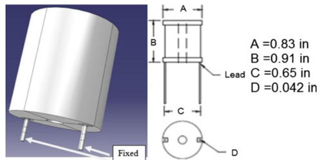
Fig. 4 Large inductor used in this study
