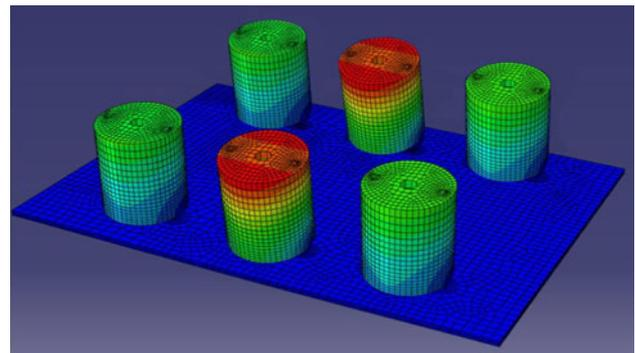
**Fig. 7** Middle inductor's first modal response
