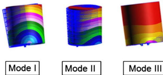
**Fig. 6** Inductor modal shapes when fixed at leads
