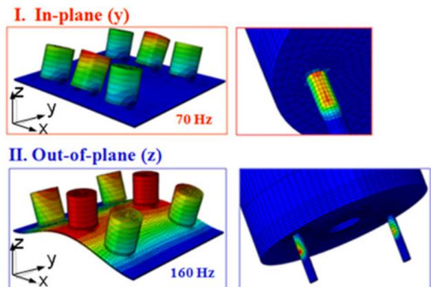
Fig. 14 Maximum stresses at component leads
