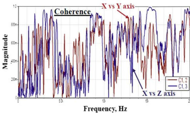
Fig. 17 Cross-axis coherence in RS shaker [7]
