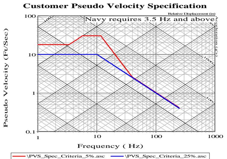
Figure 2. Specified Pseudo Velocity for a 2 second shock event
