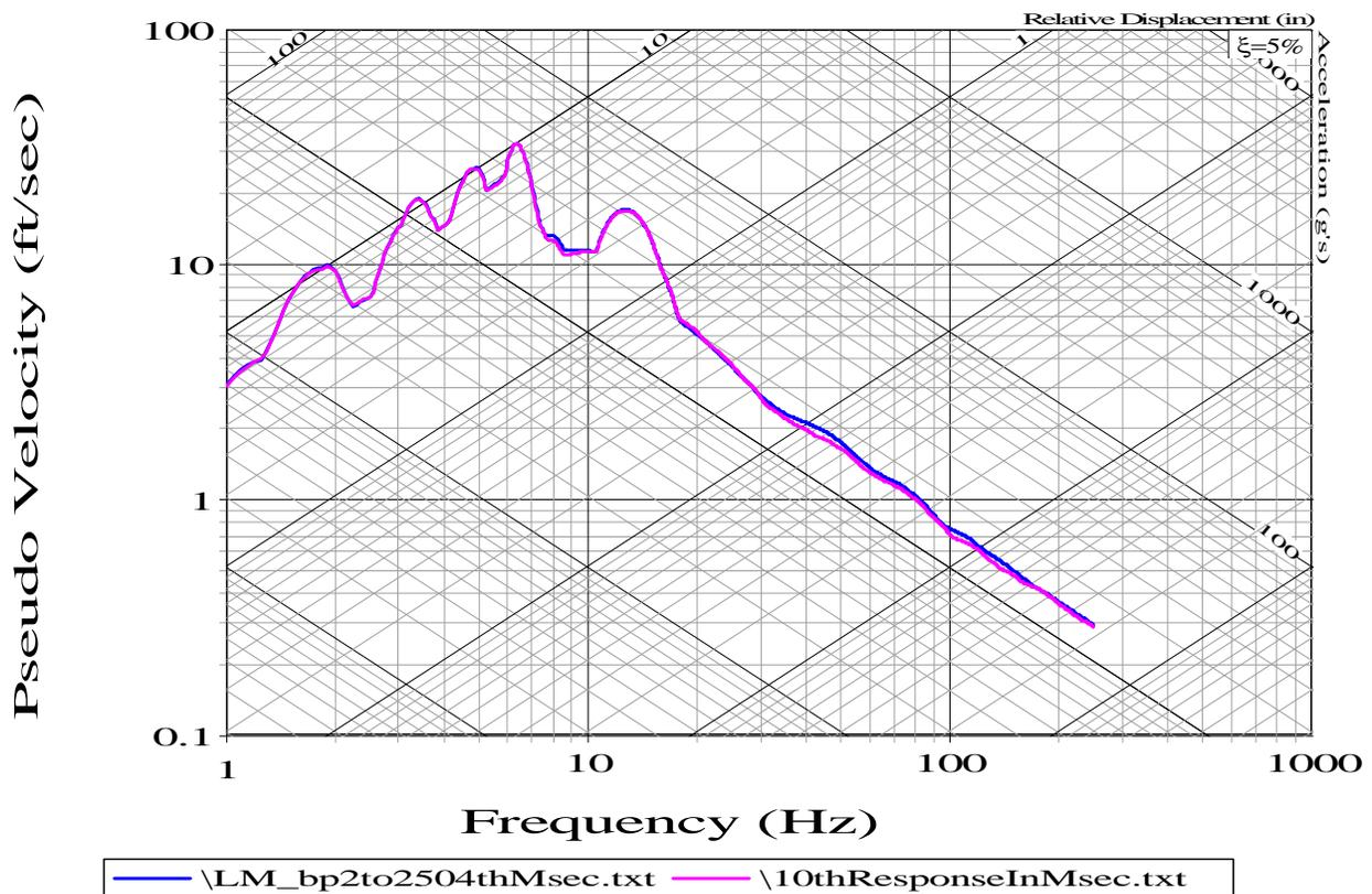
Figure 13. Pseudo Velocity of the target waveform and the SSTS response
