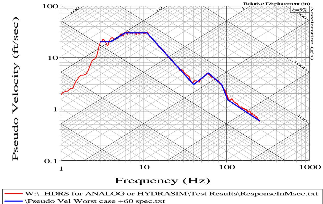
Figure 9. Pseudo Velocity Spectrum Target and Measured PSV on Demo SSTS
