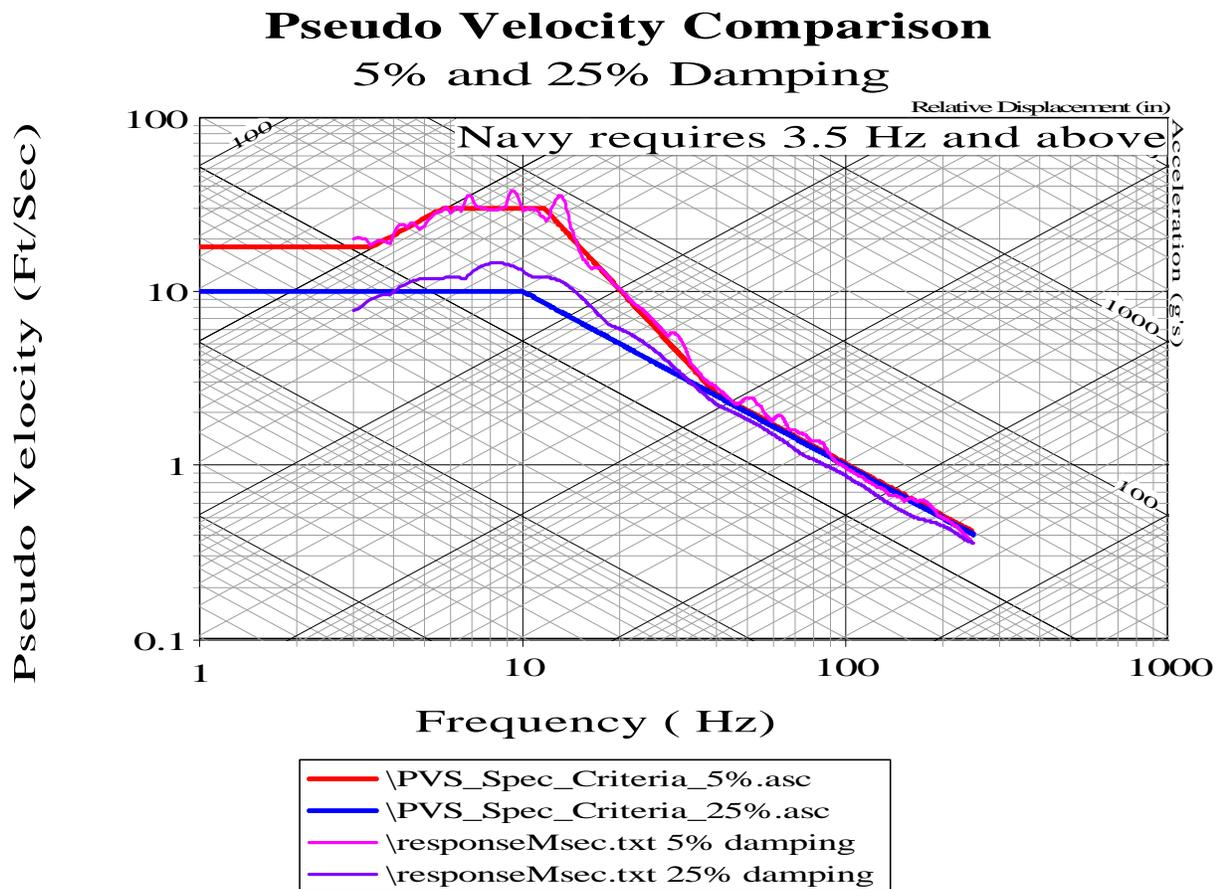
Figure 7. 5% and 25% Damping Pseudo Velocity Spectrums of Measured Acceleration with PVS criteria
