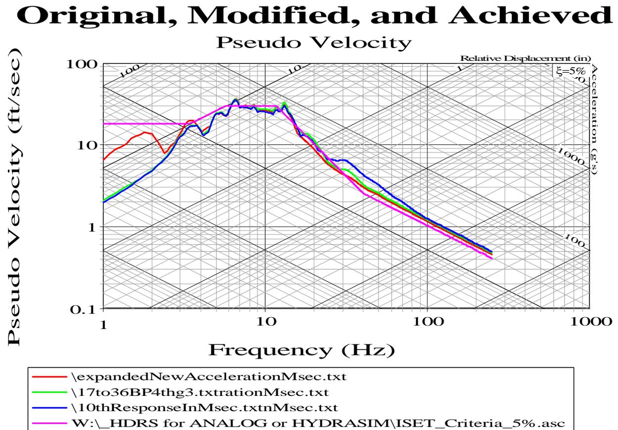
Figure 10. Pseudo Velocity of UERD preferred waveform, filtered waveform, and SSTS response
