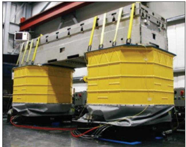
Figure 2. Dual-Cube multi-axis vibration test system.
