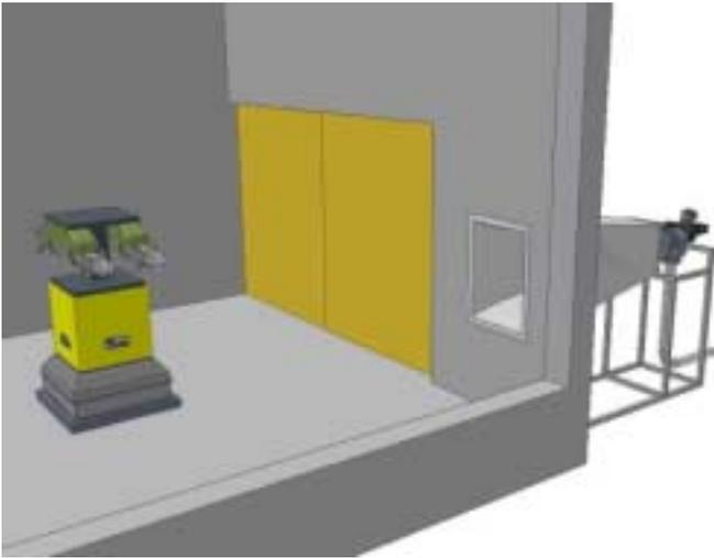
**Figure 4: Combined vibration and high-intensity acoustic test facility.**
