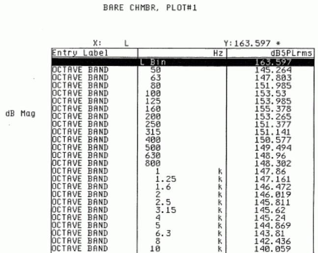
**Figure 8: One-third octave spectrum produced by Team acoustic modulator.**
