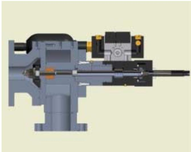
**Figure 6: Team Mark VI.2 High-intensity acoustic modulator.**
