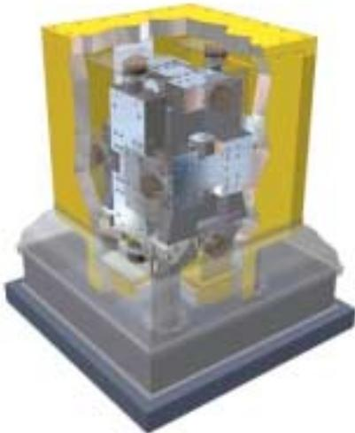
**Figure 5: Team CUBE 6-degree-of-freedom vibration test system.**
